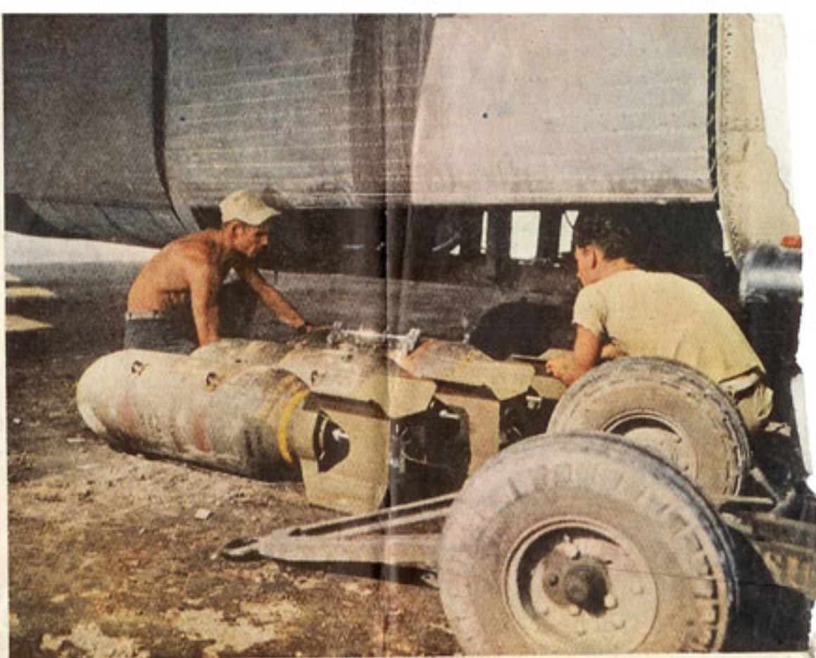
2 Fins are attached to the bombs just before they're stuffed into one of tomorrow's raiders. Bombing-up takes only twenty minutes. As it goes on, today's raiders are returning from a strike on Yap.
